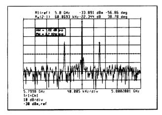
Measure AM, FM and PM: Markers read amplitude and phase of modulation sidebands, allowing for computation of AM, FM, and PM components.
