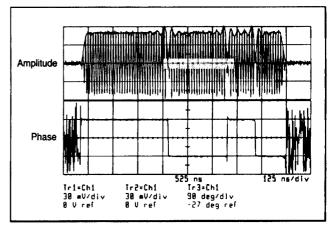
Check Barker-code response: Phase demodulation allows measurement of phase encoding within a pulse of RF. A Barker code is shown here.
