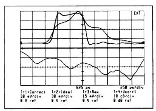
Correct for cable losses: Top half shows reference and corrected traces, which are virtually indistinguishable, as well as the wider, uncorrected pulse. Bottom trace shows the user corrections in the frequency domain.
