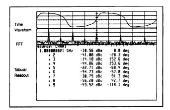
Simultaneously display time and FFT: Time and frequency domains fully characterize RF and microwave signal distortion. Tabular format allows easy comparison of results to CAE simulations.
