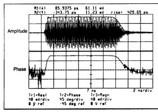
Measure fast pulses: Magnitude and phase versus time of a 12 ns wide pulse of RF. A log magnitude display is also possible.
